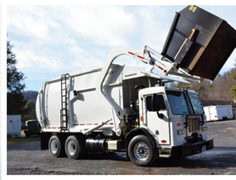
*The biodegradable soy-based hydraulic fluid is used extensively in many of the 200+ pieces of equipment used throughout the park, such as this large refuse compactor truck.*
