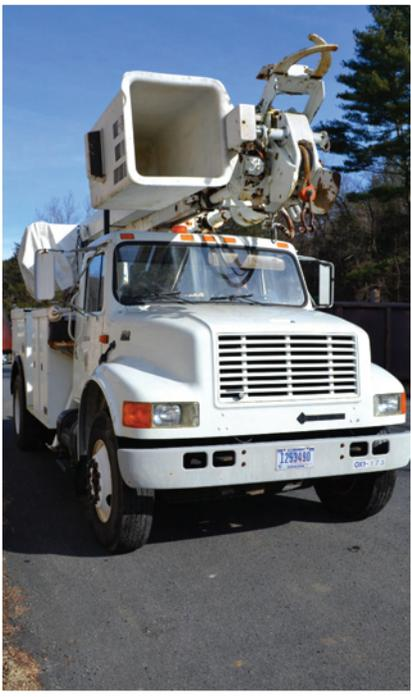
*Another large piece of maintenance equipment utilizing soy-based hydraulic fluid is this bucket lift truck used in reaching high trouble spots such as utility poles or for tree trimming.*
